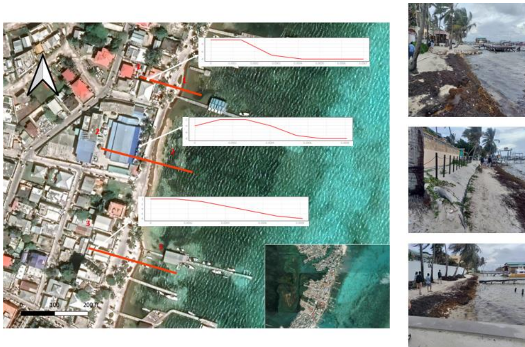
Figure 183: Central Zone – Protection walls interaction with erosion process
